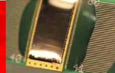
Silicon nitride photonic integrated circuit
